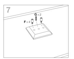
Place (F) and (G) onto side glass, fully tighten with allen key (I). Lay glass on extension with arrows facing each other.
