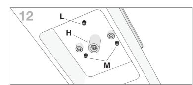
Use allen key (I) to adjust (L) clockwise to raise, counterclockwise to lower. Once leveled hand tighten (M) and fully tighten (H) with allen key (1). Repeat steps 11 & 12 on opposite side to complete assembly.
