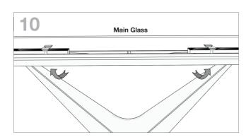
Once main glass is aligned, fully tighten (E) with allen key (I) shown in step 6.
