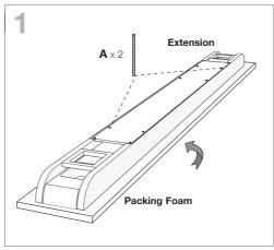
Carefully place extension on a soft surface/ packing foam. Screw on (A) diagonally on marked holes #2.
