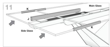
Place (K) on glass as shown. Push side glass towards main to align. Check level with (J) See step 11a for reference.
